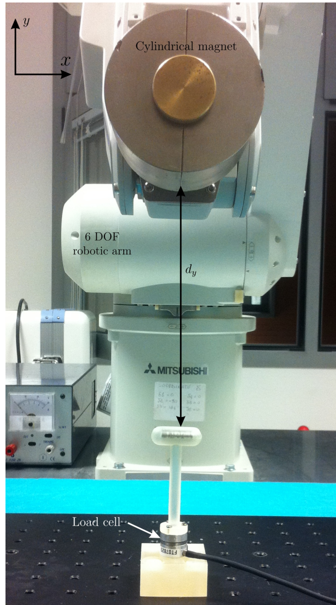
Figure A.1: Experimental setup for measuring attraction force ( F_{\vec{B}_y} ) of a typical permanent magnetic capsule locomotion system. Attraction force is then used to determine the N value for a typical magnetic capsule locomotion system.
